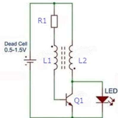
Eventually, the magnetic field can increase no further and the current flow stops and the transistor turns off. The collapsing magnetic field causes a large but brief voltage spike to be applied to the LED. This voltage causes the LED to light up briefly.
