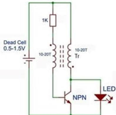
A joule thief is a self-oscillating voltage booster that is small, low-cost, and easy to build, typically used for driving small loads, such as driving an LED using a 1.5 volt battery.
