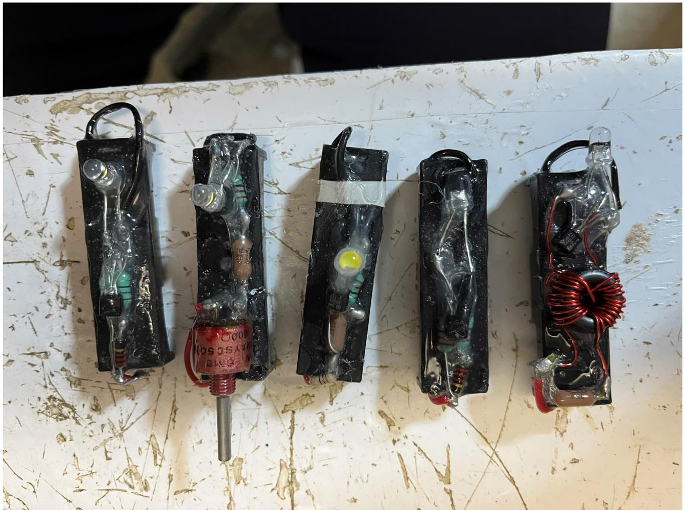
This photo shows a Joule Thief prototype with a brightness control mounted in a medicine container for use as a nightlight.
