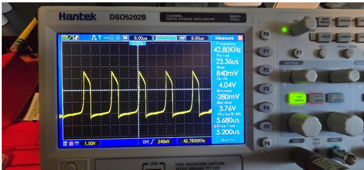
With 1.0 volt applied to the Joule Thief, the frequency is 42,800 cycles per second, which produces an output voltage of 4.04 volts. One volt in, yields four volts out.
