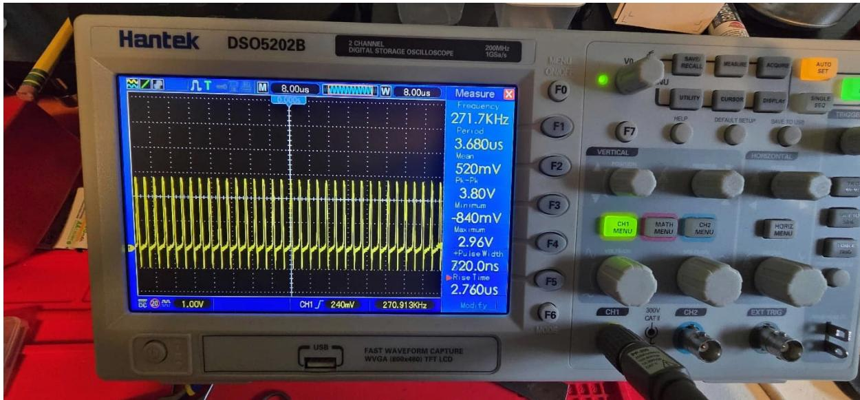
With 0.5 volt applied to the Joule Thief, the frequency is 271,700 cycles per second producing an output voltage of 3.8 volts. One half volt in, 3.8 volts out.
