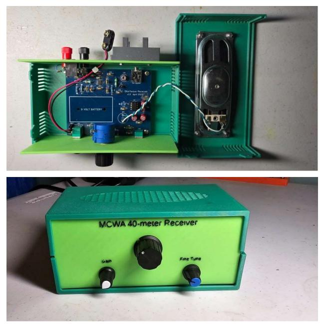
These photos shows a receiver with modifications and its 3D printed case.
