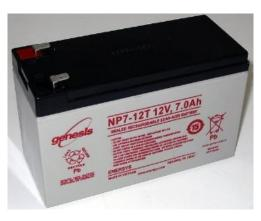
Typical Sealed Lead Acid battery often incorrectly called Gel-Cell. Typical life is about 3-5 years, after that they become unreliable at holding charge.
